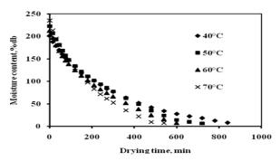
Figure 1. Variation of moisture content (dry basis) with drying time of stone apple slices dried by convective drying at different temperatures
